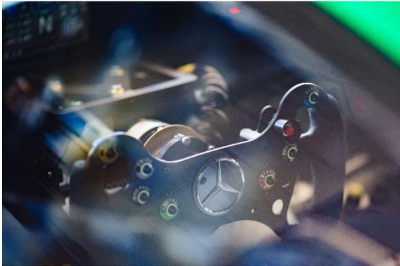
*Thanks to Space Drive, the Mercedes-AMG GT3 #18 manages without any mechanical connection between the steering unit and Steering gear, Photo: GruppeC Photography*
