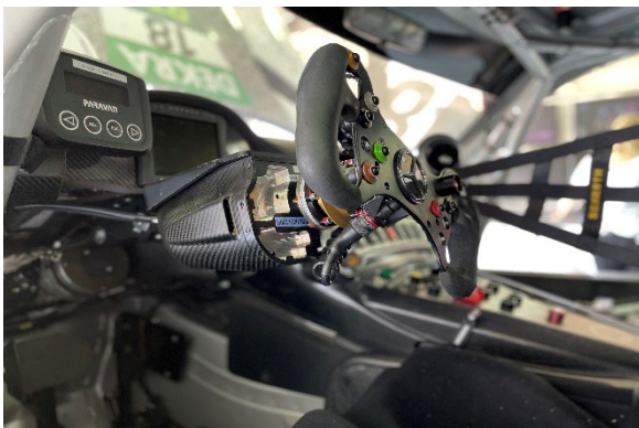
The Mercedes-AMG GT3 does without any mechanical connection between the steering unit (force feedback) and the steering gear, Photo: Schaeffler-Paravan
