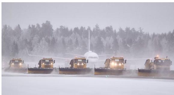
*Thanks to Space Drive, a wide variety of applications can be realized, for example platooning applications. Up to ten snow removal machines can be guided by a lead vehicle. Photo: Overassen*
